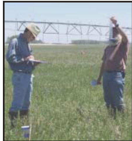
NRCS technicians measure water applied by the center pivot this effort is part of the overall cooperative Irrigation Water Management Program by the Eden Valley Irrigation and Drainage District and NRCS.
